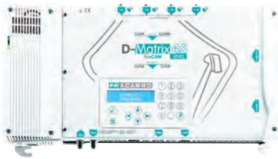
**Compact headend** to distribute up to **20-25** digital satellite DVB-S/S2 channels (FTA or ENC) coming from 4 different satellite transponders on 4 DVB-T or DVB-C output muxes.
