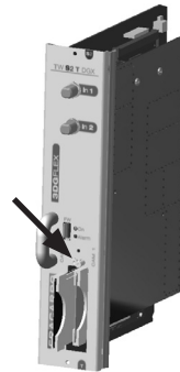
To remove the CAM, press the corresponding button
