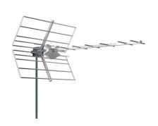
**UHF band** Yagi aerial complete with F connector, **tube reflectors** and **double filtering**, which combines the 5G and 4G LTE frequencies selection given by the **elements geometry** to the **5G filter integrated** in the radiator dipole.
