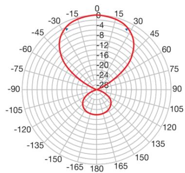
**Ganancia (x: frecuencia MHz, y: ganancia ISO dBi) y radiación (@600MHz)**
