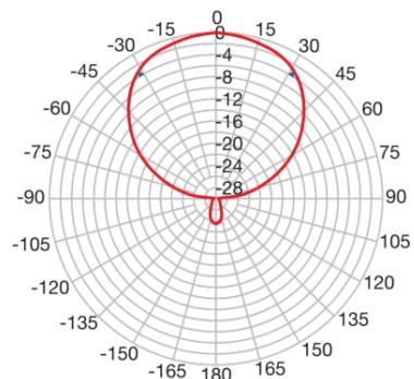
**Gain (x : fréquence MHz, y : gain ISO dBi) et diagramme (@600MHz)**
