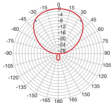
**Gain (x : fréquence MHz, y : gain ISO dBi) et diagramme (@600MHz)**
