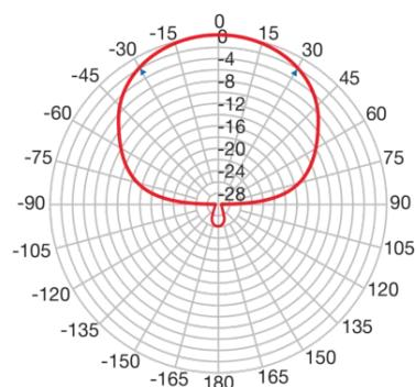
**Ganancia (x: frecuencia MHz, y: ganancia ISO dBi) y radiación (@600MHz)**
