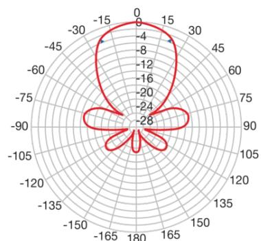
**Ganancia (x: frecuencia MHz, y: ganancia ISO dBi) y diagrama de radiación (@862MHz)**
