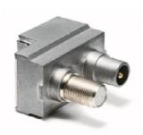
Pass through outlet with 10dB attenuation; 2 demixed outputs with IEC Male connector for TV band (47-862MHz) and F Female connector for Satellite band (950-2400MHz).
