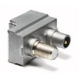
Pass through outlet with 5dB attenuation; 2 demixed outputs with IEC Male connector for TV band (47-862MHz) and F Female connector for Satellite band (950-2400MHz).
