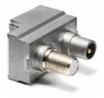
**Terminal outlet; 2 demixed outputs** with IEC Male connector for TV band (**47-862MHz**) and F Female connector for Satellite band (**950-2400MHz**).
