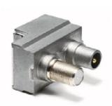
Pass through outlet with 14dB attenuation; 2 demixed outputs with IEC Male connector for TV band (47-862MHz) and F Female connector for Satellite band (950-2400MHz).
