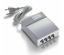
1-input (VHF+UHF) indoor amplifier with RC and 2 outputs, 20dB gain and up to  $108dB\mu V$  output level on UHF band, level adjustment (15dB) and low noise figure.
