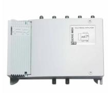
2-input (RC+FM+VHF+UHF, SAT) indoor amplifier with 37-43dB uptilted gain and up to 120dBµV output level on SAT band, gain adjustment (15dB) and low noise figure.
