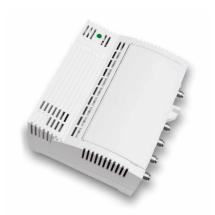
MBK Line Multiband TV indoor amplifier to amplify and mix signals from one or more aerials; with F connectors, separate amplification and independent level adjustment for each input and low noise figure. 790MHz 4G LTE integrated filter.
