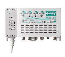
4-input (III+DAB, IV, V, UHF) multiband TV indoor amplifier with 35dB gain and up to  $120dB\mu V$  output level on UHF band, separate amplification with independent level adjustment (20dB) for each input and low noise figure. 790MHz 4G LTE integrated filter.
