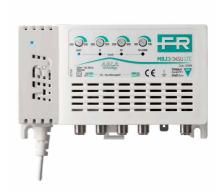
4-input (III+DAB, IV, V, UHF) multiband TV indoor amplifier with 35dB gain and up to  $120dB\mu V$  output level on UHF band, separate amplification with independent level adjustment (20dB) for each input and low noise figure. Version available with special tuning on the cut between band IV and V and 790MHz 4G LTE integrated filter.
