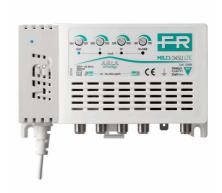
4-input (III+DAB, IV, V, UHF) multiband TV indoor amplifier with 20dB gain and up to 115dBμV output level on UHF band, separate amplification with independent level adjustment (20dB) for each input and low noise figure. Version available with special tuning on the cut between band IV and V and 790MHz 4G LTE integrated filter.
