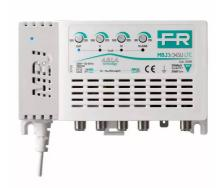
1-input (III+DAB+IV+V) multiband TV indoor amplifier with 25dB gain and up to  $115dB\mu V$  output level on UHF band, separate bands amplification with independent level adjustment (20dB) for each band and low noise figure. 790MHz 4G LTE integrated filter.
