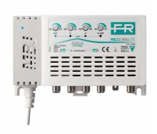
3 input (FM+III+DAB, UHF) multiband TV indoor amplifier with 32dB gain and output level up to 120dBμV in UHF band, separate amplification, independent level adjustment (20dB) for each input and low noise figure. Built-in 694MHz 5G and 4G LTE filter.
