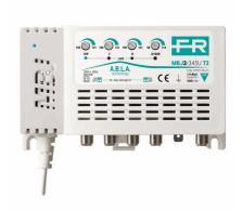
4-input (III+DAB, IV, V, UHF) multiband TV indoor amplifier with 35dB gain and up to  $120dB\mu V$  output level on UHF band, separate amplification with independent level adjustment (20dB) for each input and low noise figure. Version available with special tuning on the cut between band IV and V and T2 technology with UHF cut band for LTE 4G @790MHz and 5G @694MHz.
