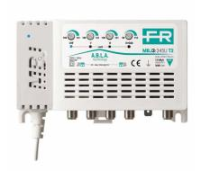
4-input (III+DAB, IV, V, UHF) multiband TV indoor amplifier with 35dB gain and up to 120dBμV output level on UHF band, separate amplification with independent level adjustment (20dB) for each input and low noise figure. T2 technology with UHF cut band for LTE 4G @790MHz and 5G @694MHz.
