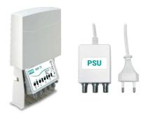
2-input (III+DAB, UHF) mast amplifier with 42dB gain and up to 116dBµV output level on UHF band, separate VHF/UHF amplification with independent gain adjustment (0-15dB) for each input and low noise figure. T2 technology with UHF cut band for LTE 4G @790MHz and 5G @694MHz. **Power supply included in the package.**
