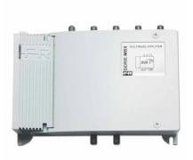
1-input (RC+VHF+UHF+SAT) indoor amplifier with 45dB gain and up to 127dBµV output level on UHF band, separate amplification with independent gain and tilt adjustment (20dB) for TV and SAT bands and low noise figure.
