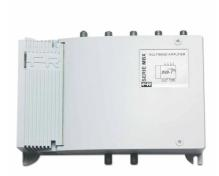
Central unit with 1 input (RC+VHF+UHF) self-powered indoor with 42dB gain and output level up to 127dBµV in UHF band, gain and slope adjustment (20dB) and low noise figure.
