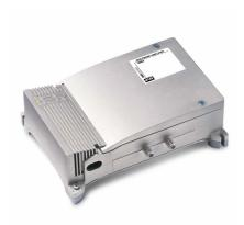
4-input (III+DAB, IV, V, UHF) multiband TV indoor amplifier with 40dB gain and up to  $130dB\mu V$  output level on UHF band, separate amplification with independent level adjustment (20dB) for each input and low noise figure.
