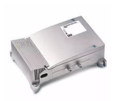
4-input (III+DAB, IV, V, UHF) multiband TV indoor amplifier with 31dB gain and up to  $125dB\mu V$  output level on UHF band, separate amplification with independent level adjustment (20dB) for each input and low noise figure. 790MHz 4G LTE integrated filter.
