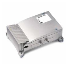
4-input (FM, III+DAB, UHF, UHF) multiband TV indoor amplifier with 43dB gain and up to  $125dB\mu V$  output level on UHF band, separate amplification with independent level adjustment (20dB) for each input and low noise figure. 790MHz 4G LTE integrated filter.
