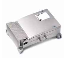
4-input (FM, III+DAB, UHF, UHF) multiband TV indoor amplifier with 31dB gain and up to  $125dB\mu V$  output level on UHF band, separate amplification with independent level adjustment (20dB) for each input and low noise figure. 790MHz 4G LTE integrated filter.
