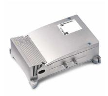
4-input (III+DAB, IV, V, UHF) multiband TV indoor amplifier with 31dB gain and up to  $125dB\mu V$  output level on UHF band, separate amplification with independent level adjustment (20dB) for each input and low noise figure. Version available with special tuning on the cut between band IV and V and 790MHz 4G LTE integrated filter.
