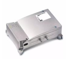
4-input (FM, III+DAB, UHF, UHF) multiband TV indoor amplifier with 43dB gain and up to  $125dB\mu V$  output level on UHF band, separate amplification with independent level adjustment (20dB) for each input and low noise figure. 694MHz 5G and 4G LTE integrated filter.
