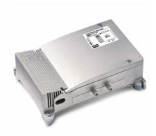
4-input (III+DAB, IV, V, UHF) multiband TV indoor amplifier with 31dB gain and up to 125dBμV output level on UHF band, separate amplification with independent level adjustment (20dB) for each input and low noise figure. T2 technology with UHF cut band for LTE 4G @790MHz and 5G @694MHz.
