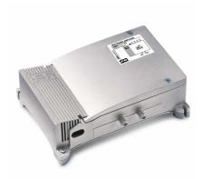
4-input (FM, III+DAB, UHF, UHF) multiband TV indoor amplifier with 43dB gain and up to 125dBμV output level on UHF band, separate amplification with independent level adjustment (20dB) for each input and low noise figure. T2 technology with UHF cut band for LTE 4G @790MHz and 5G @694MHz.
