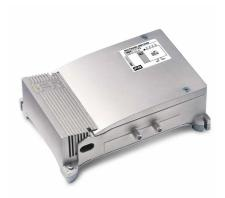
1-input (III+DAB+UHF) multiband TV indoor amplifier with 31dB gain and up to  $125dB\mu V$  output level on UHF band, separate amplification with independent level adjustment (20dB) for each band and low noise figure. T2 technology with UHF cut band for LTE 4G @790MHz and 5G @694MHz.
