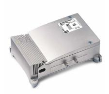
Central unit with 4 inputs (FM, III+DAB, UHF, UHF) self-powered indoor with 43dB gain and output level up to 125dBµV in UHF band, separate band amplifications, independent gain adjustments (0-20dB) for each input and low noise figure. Built-in 5G and 4G LTE 694MHz filter and UK G-type plug.
