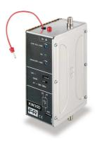
Wideband amplifiers with push-pull technology capable of amplifying the entire 47-862 MHz band. Equipped with one input and one output, they are used to amplify the signal coming from a KF filter battery or other modules (receivers, modulators, etc.).
