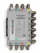
4-input cascadable multiswitch with 6 output taps and 8dB attenuation.
