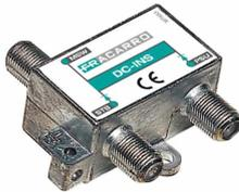
Current inserter with protection of DiSEqC tones generated by the STBs with a maximum of 450mA current throughput. It can work both with SCR (190mA) or SCD2 dCSS (350mA).
