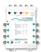
**5-input compact** multiswitch with **8 output taps**; active gain on TV and Satellite bands and compatibility with QUAD and QUATTRO LNBs.
