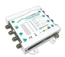
Compact SCD2 (dCSS) multiswitch ADAPTOR; 4 inputs with CAG, 4 output taps: 2 Legacy (traditional) and 2 with 16 frequencies each; entirely fed by the receivers. SKY UK frequencies.
