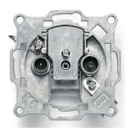
wall mount terminal rounded outlet; 2 demixed outputs with IEC Female connector for TV band (47-862MHz) and IEC Male connector for Satellite band (950-2400MHz). The outlet demixes input TV+SAT combined signal to 2 different output connectors.
