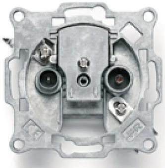
wall mount pass through rounded outlet with 6dB attenuation; 2 demixed outputs with IEC Female connector for TV band (47-862MHz) and IEC Male connector for Satellite band (950-2400MHz). The outlet demixes input TV+SAT combined signal to 2 different output connectors.
