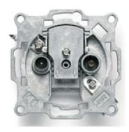
wall mount pass through rounded outlet with 6dB attenuation; 2 demixed outputs with IEC Female connector for TV band (47-862MHz) and IEC Male connector for Satellite band (950-2400MHz). The outlet demixes input TV+SAT combined signal to 2 different output connectors.
