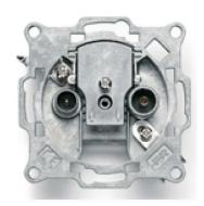
wall mount pass through rounded outlet with 18dB attenuation; 2 demixed outputs with IEC Female connector for TV band (47-862MHz) and IEC Male connector for Satellite band (950-2400MHz). The outlet demixes input TV+SAT combined signal to 2 different output connectors.
