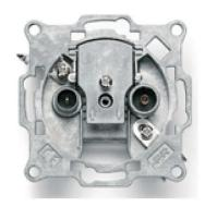
wall mount pass through rounded outlet with 22dB attenuation; 2 demixed outputs with IEC Female connector for TV band (47-862MHz) and IEC Male connector for Satellite band (950-2400MHz). The outlet demixes input TV+SAT combined signal to 2 different output connectors.
