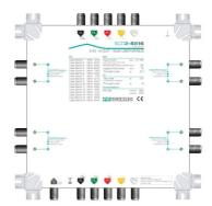
5-input cascadable SCD2 (dCSS) multiswitch with CAG; 8 output taps with 16 frequencies each and operating mode autodetection, entirely fed by the receivers. SKY Italian frequencies.
