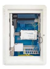
Apartment box (54 modules) to be walled in, complete with 2 DIN bars with associated Router hookups, active patch-cord RJ45 apparatus for data and SC/APC patch cords for connections to STOA (dimensions 455x136x610mm including frame, recessed 592x427x100)
