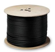
Outdoor CAT 6 network cable with black PE sheathing, 500-m skein consisting of 4 balanced 100 Ohm pairs with AWG 24 flexible red copper conductors. Features meet the requirements of Cat. 6 Class E up to 250Mhz according to ANSI/TIA 568.2-D and ISO/IEC 11801 standards. Suitable for Gigabit Ethernet (IEEE 802.3ab) applications.
