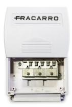
**4-output pole-mounting clamp splitter** of the PAM series in the TV and Satellite bands (**5-2400MHz**) on **BOM box** for external use with **included clamp for pole-fixing**.
