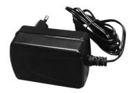
**12V 1.5A power supply** with **male jack connector** (2.1 x 5.5 x 12mm; inner positive, outer negative) and European plug.
