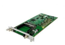
**GX-4S2CI-BP-01** module is equipped with two RF coaxial Satellite inputs and two PCMCIA Common Interface slots. The module is able to tune up to **four DVB-S/S2/S2X satellite transponders** (two transponders for every single RF coaxial input), decrypt the scrambled programs through the C.I. slots and share and pool the contents to the **GALAXIA** main chassis.
